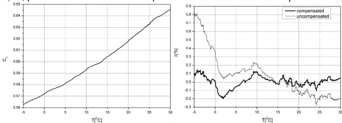
Fig. 2. Normalized channel 3 output as a function of the reference temperature (left), and comparison of relative errors of uncompensated and compensated FEFOS sensed currents (right)
