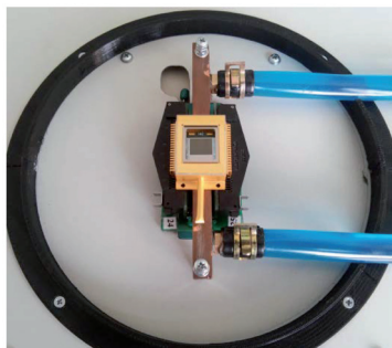
Fig. 2. Measuring system in general and an example of how a 640x512 EMCCD chip is connected to the system
